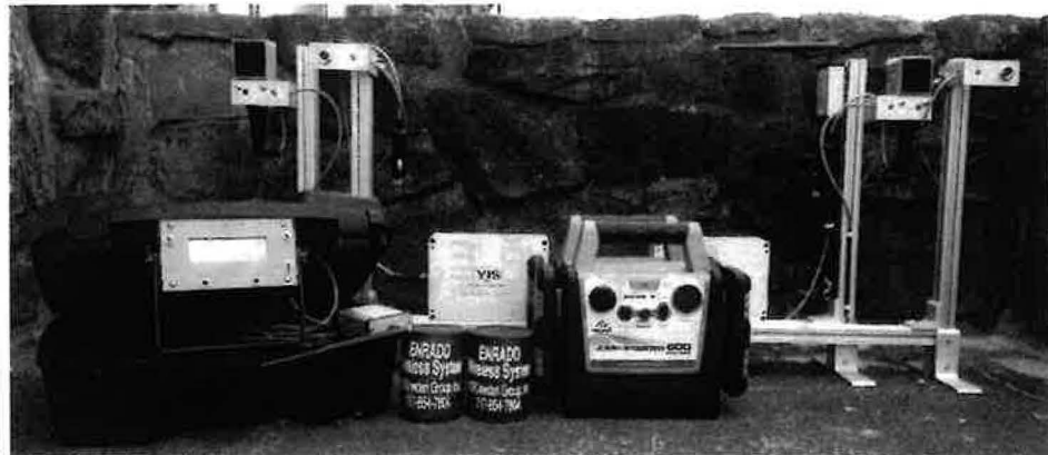
ENRADD Wireless System – Electronic device that calculates speed between two sensors
