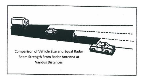
Echoing the challenges of correct target vehicle identification, The Northwestern University Traffic Institute suggests that the radar operator should use a minimum of three seconds in vehicle spacing, and that a radar operator "should not attempt to take readings where vehicles are spaced less than three seconds apart or when vehicles are traveling side by side."
